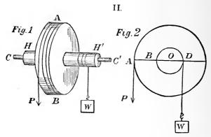
97. Description of Wheel and Axle. This machine consists of a wheel AB, and a cylinder or axle HH'; both turning round the same axis. The points C,C', are placed on bearings so as to allow of motion round the common axis. The power is applied at the circumference of the wheel, generally by a cord wrapped round it, as in the figure, and the weight is attached to a cord coiled round the axle in the contrary direction, so that when P descends, W ascends, and vice versa.
